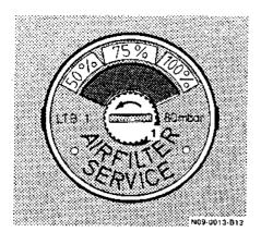
230 GEMaintenance indicator in the air filter1 Reset button
